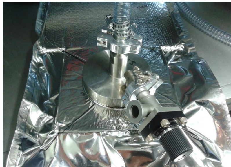
Figure 4: Specimen with the leak-tight connector and a connector support inside one half and a standard fumed silica core inside the other part of the panel
