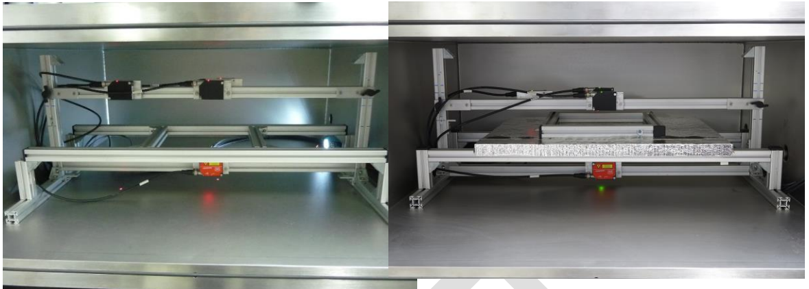
Figure 11: Modified Setup with square-shaped restriction of the measurement are on both sides of the specimen
