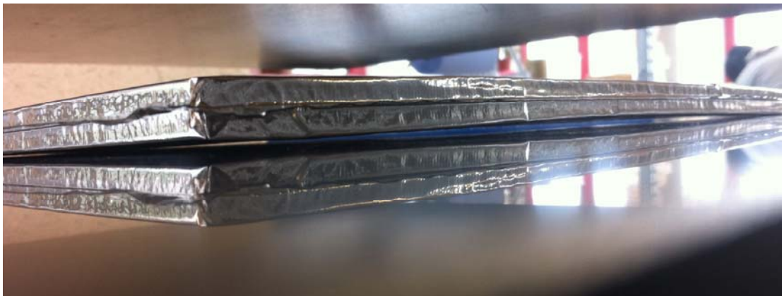
fig. 6 VIP with silica core and without surface seam, size 300 mm x 300 mm x 10 mm, in the testing machine before applying the initial force
