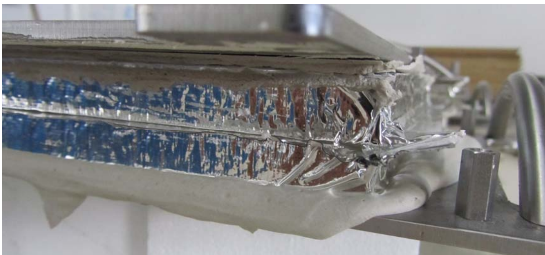
fig. 25 Specimen preparation of a vacuum insulation panel, 30 mm, silica core. Specimen with gypsum coating on both sides
