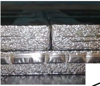
Figure 5: Situation B2 single joint with seal in one layer. A typical gap between the VIP cores can be seen at this 40mm + 40mm situation.
