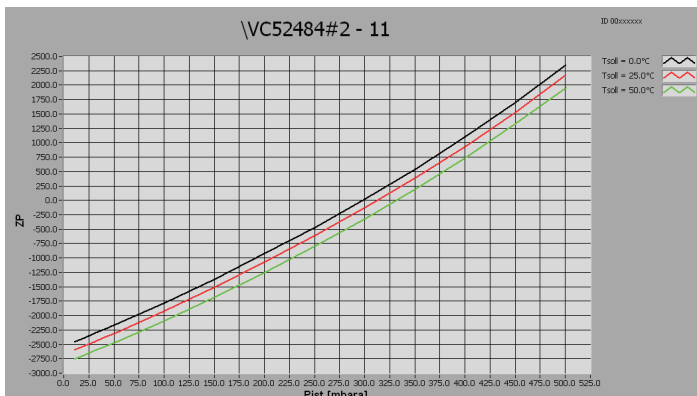
Fig. 7 Typical pressure characteristics (Pist: applied pressure, ZP: raw values)
