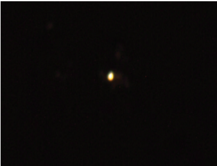
Fig. 1. Optical microscope (back lit) of a barrier where there was a physical hole.
