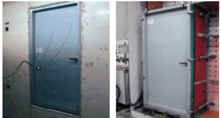
Fig. 9: Prototype of insulation door applying the vacuum insulation materials
