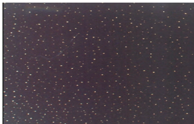
Fig.3 Starry Night – A photograph of Al layer deposited on thin PET film and containing tens of microns size pinholes. In high quality metallized films the overall surface area covered by the pinholes is less than 2%. However they are considered to be the main route for oxygen and nitrogen permeation.
