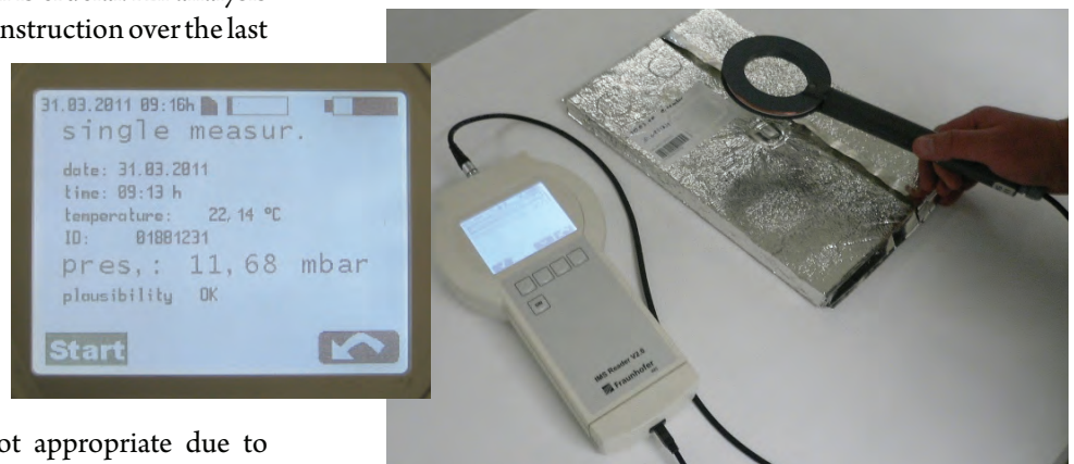
Fig. 1 Readout of the inside pressure and temperature of a VIP
