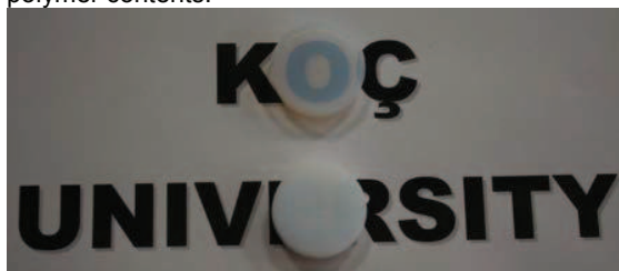
Fig 2: Silica aerogel samples with 17 %wt. (top) and 50 %wt. (bottom) PDMS(OH) content.
