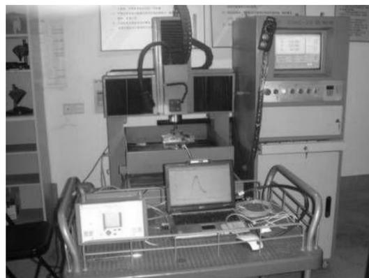
**Fig. 3** Drilling CFRP laminate equipments
