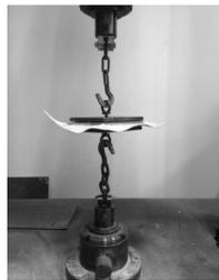
Fig. 2 Pullout testing for VIP
