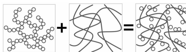
Fig. 3 Schematic drawing of the synthesis of a fiber reinforced HSNS composite
