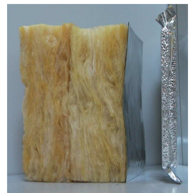
Comparison of thickness of VIP (right) and glass wool fibres (left) with similar thermal resistance.
