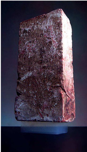
Figure 2: Silica aerogel with 30-35% solid content is a strong material. By increasing the solid content up to 60% the strength will be improved.
