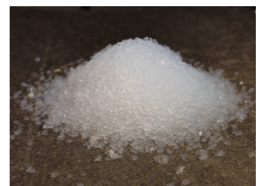
Aerogel granulate has a low thermal conductivity due to its nanoporous structure.
