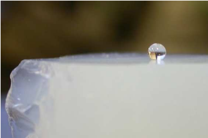
Figure 4: Picture of a water droplet on a hydrophobic aerogel
