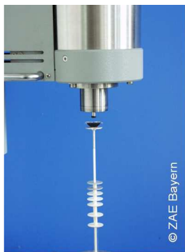
THERMAL Analysis - Experimental Equipment - ZAE Bayern: Sample holder of differential scanning
