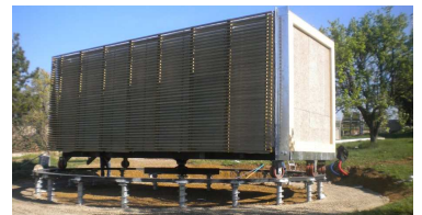
New design of PASLINK testcell in Florence
