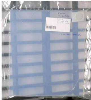
Fig 3: Transparent VIP with Silica Aerogel core
