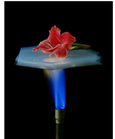
Figure 7 - Silica aerogel has excellent thermal properties. The fire retardant (inherent to silica-based composition) are intrinsic properties of an aerogel
